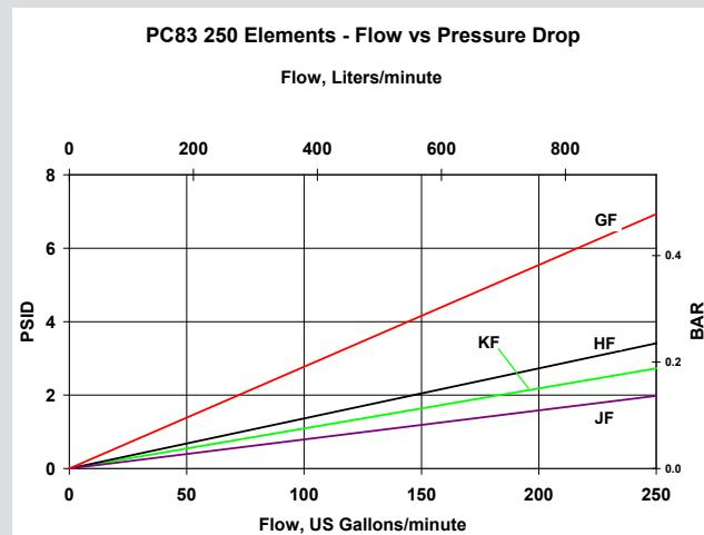
Pressure drop curves are based on 150 SUS (32 cSt) petroleum base hydraulic fluid of 0.9 S.G.
